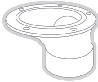
An offset closet ring allows the opening of pipe to be altered and alignment with the pipe already in place.
