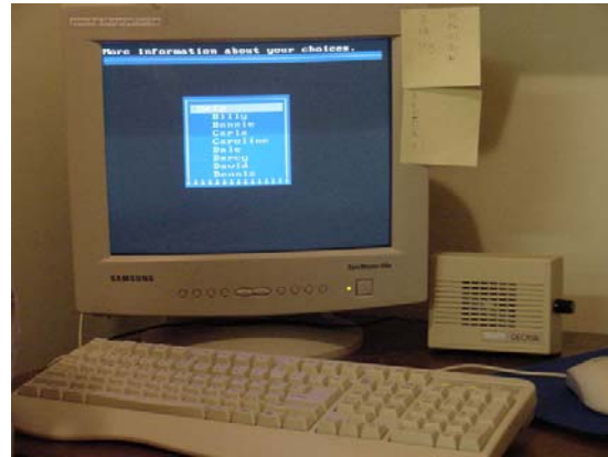
The SARAW program loaded on a computer. The DECtalk speech synthesiser module is on the right.
